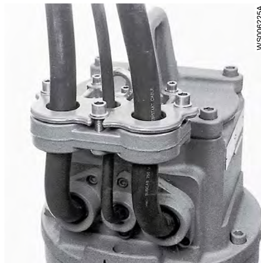
Figure 19: Cable holder. Pumps equipped with MAS 801 do not have the auxiliary cable.
